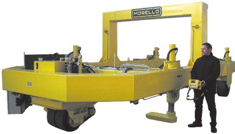
SGAI - VS E 20/2 Capacity load 20 t Containers lifting and translation
