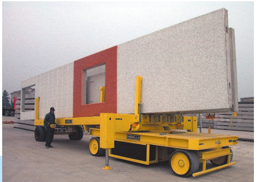
SGAI – VS E 35/2 Load capacity 35 t Tow capacity 35 t Prefabricated building handling max 70 t of weight
