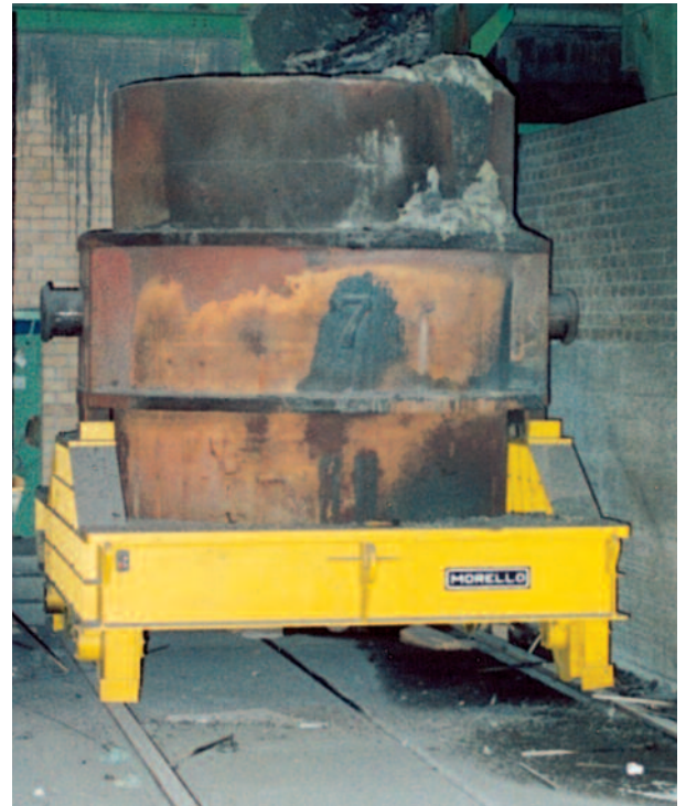
SBR 4R 140/2 Capacity load 140 t Iron ladles handling
