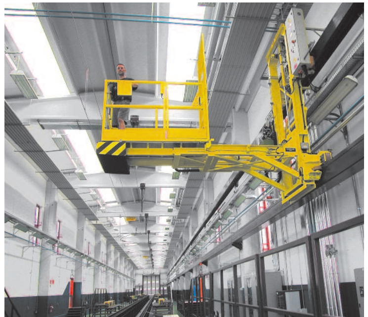
Handling system for testing sector Capacity load 250 kg Upstroke 1000 mm Transversal run 1600 mm Longitudinal run 118 m
