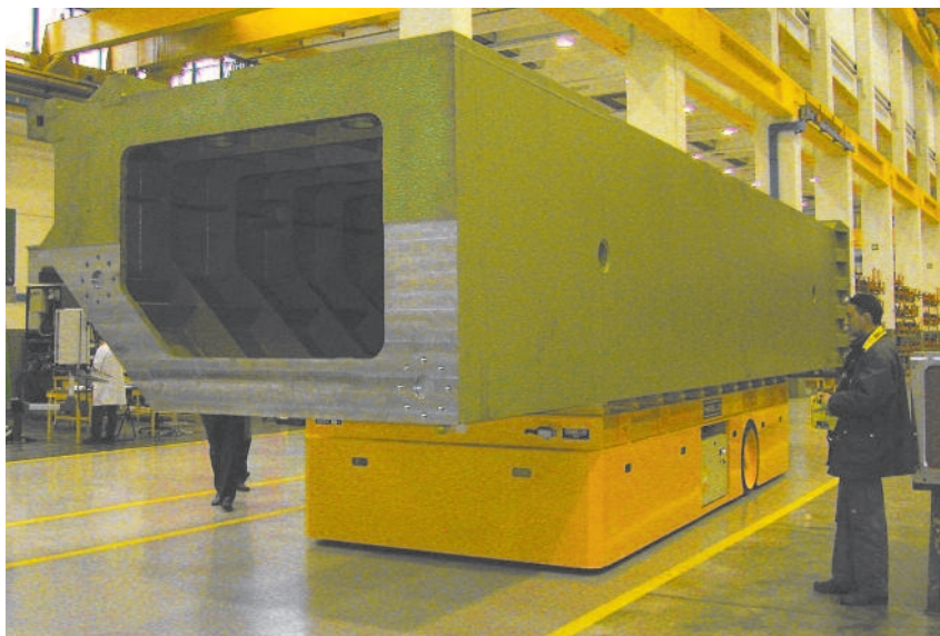
SGAI - VS/VSP1 60/2 60 t – 6000 x 2400 mm Steel structures handling
