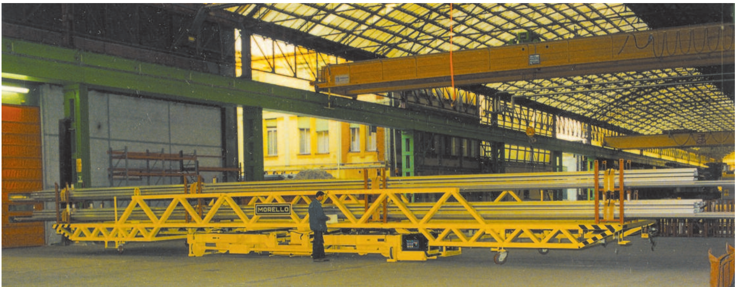
SBA 4 + 4R 10/2 10 t – 18000 x 3400 mm Aluminium section bar with rotation of 180° of the loading platform and translation on orthogonal rails
