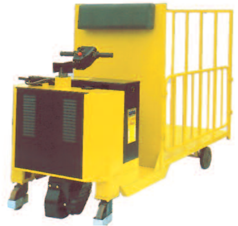
SGAM - 2/2 2 t - 1200 x 800 mm Various material handling
