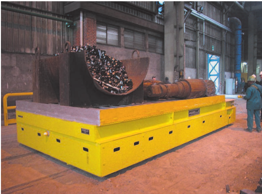
SBA 4R 50/2 with suspensions 50 t – 5000 x 3000 mm Iron metallurgy products handling
