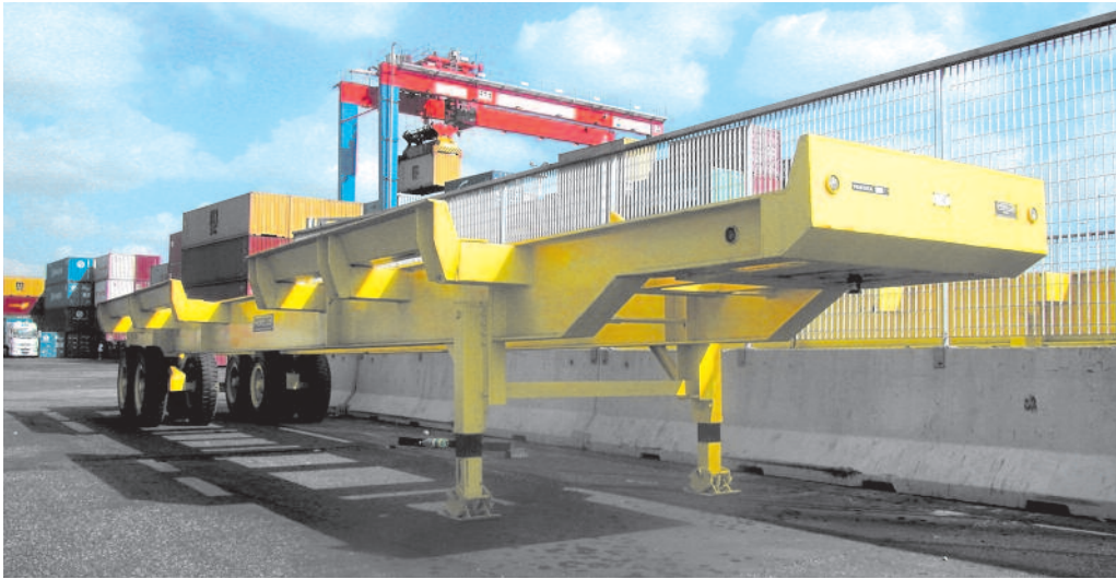
Skeletal trailer STP2 60/2 Capacity load 60 t Containers handling of 45' – 40' – 20'
