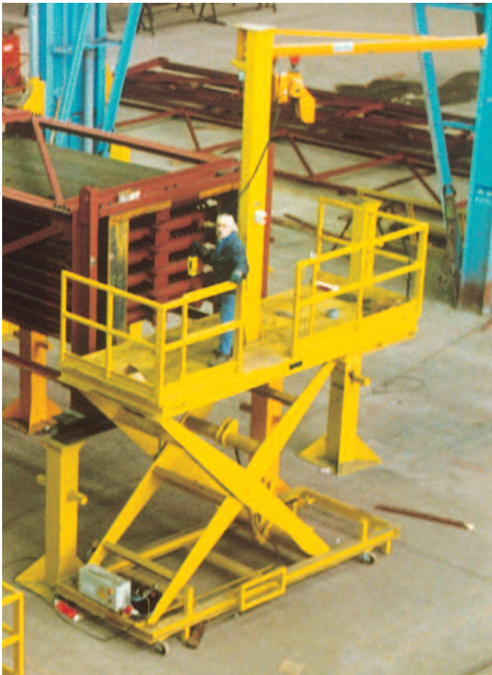
PE F 1/X 1 t – 4000 x 1500 x 800 (3000) mm Personnel and components handling of industrial boilers
