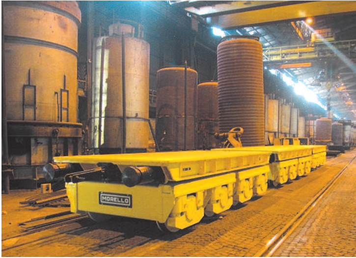
FB 8R 180/2 with suspensions 180 t – 5200 x 2200 mm Coils handling
