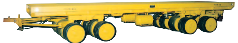
VCP3 125/4 125 t – 8000 x 2500 mm Steel plant machines handling
