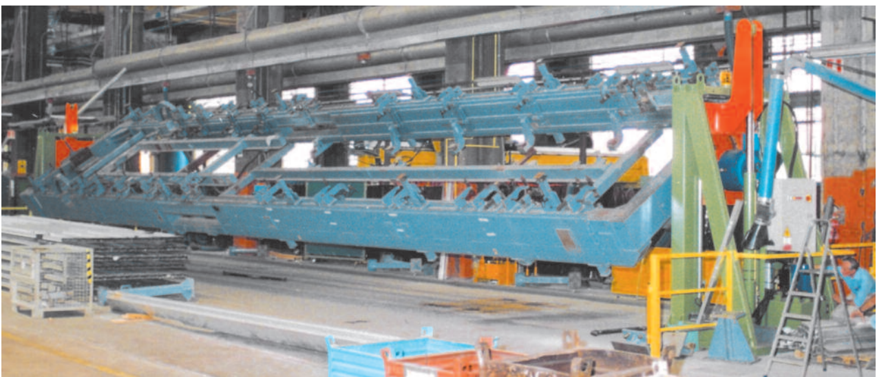
RA 30/360 Capacity load 30 t 360° equipments tipper
