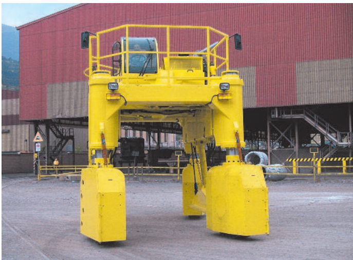
SGD VC E 30/2 Capacity load 30 t Iron and steel products translation and lifting
