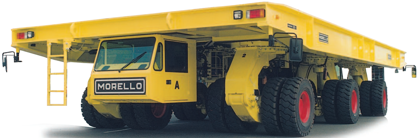
SGD VCP4 E 150/3 150 t – 12000 x 6000 x 1650 (2250) mm Naval structures handling
