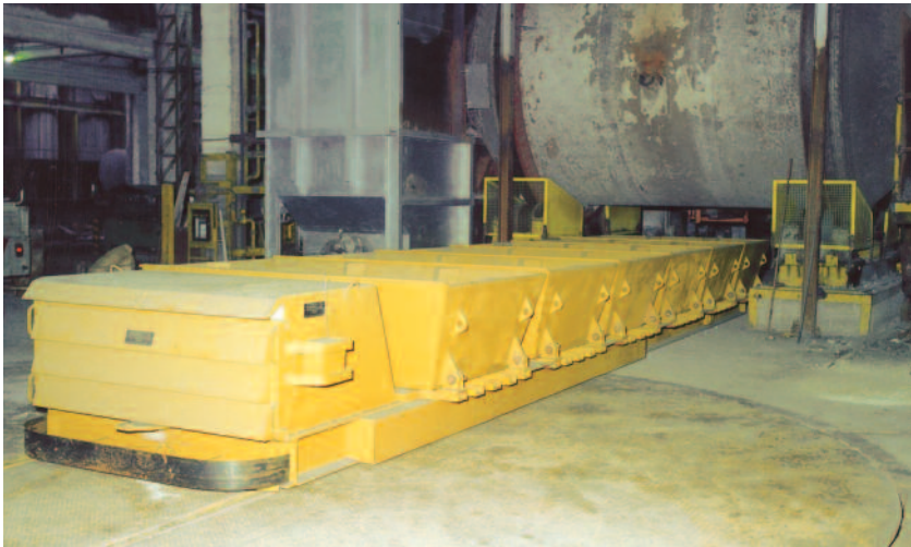
SBA 6R 20/3 with turntable Capacity load 20 t Tanks handling containing aluminium exhaust salt
