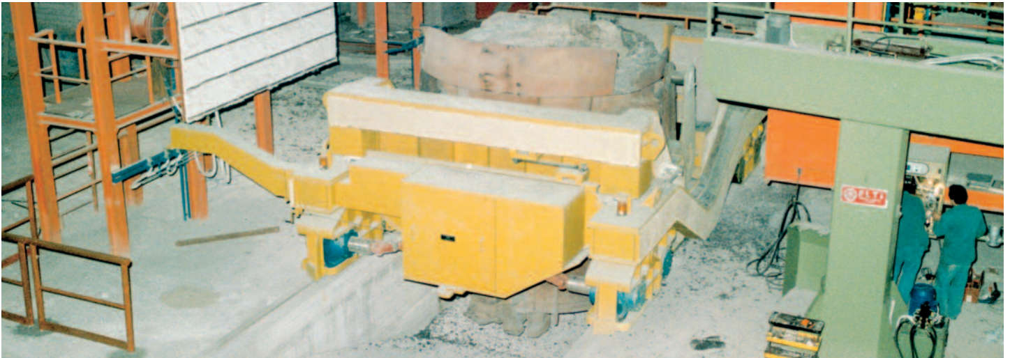
SBR 8R 120/4 Capacity load 120 t Iron ladles handling
