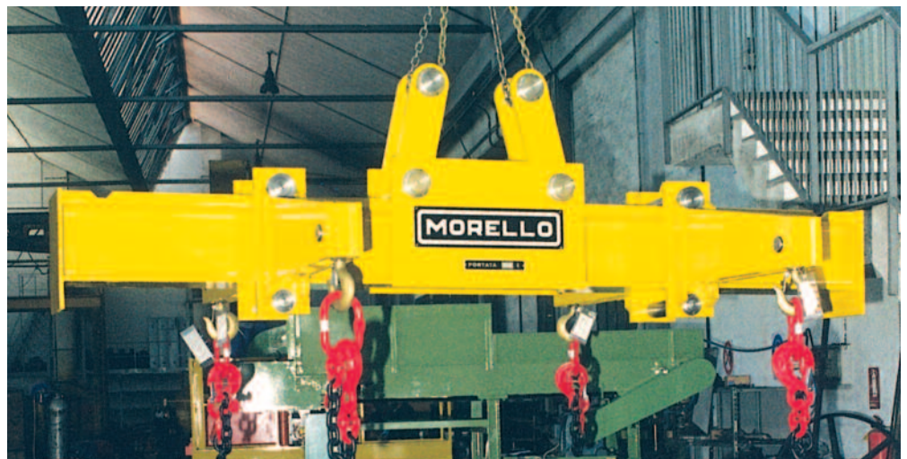
Cross members for lifting Capacity loads up to 40 t At fixed and adjustable axle base
