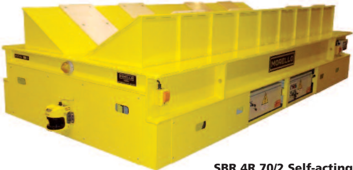
SBR 4R 70/2 Self-acting 70 t – 4600 x 2000 mm Coils handling
