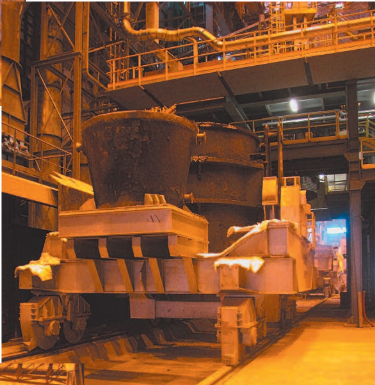
SBR 8R 440/4 Capacity load 440 t with weighing system Ladles steel mill handling
