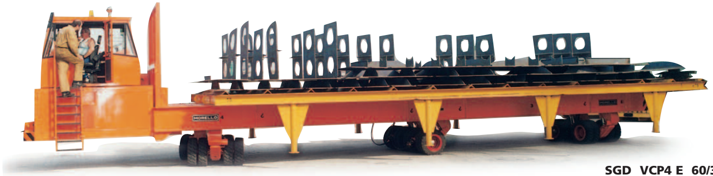
SGD VCP4 E 60/3 60 t – 14000 x 3500 x 1000 (1600) mm Pallets handling
