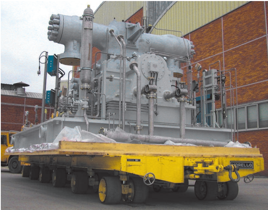
VCP4 100/6 100 t – 11000 x 3200 mm Turbines handling
