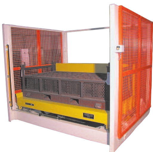
RC 3/90 3 t – 1200 x 650 x 2000 mm 90° tipper for foundry boxes
