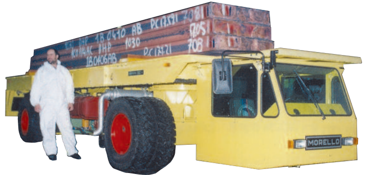
SGD VC 40/2 40 t – 7500 x 2200 x 1000 mm Thick slabs handling
