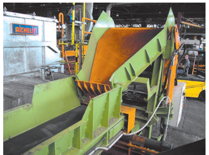
RC 3/180 with conveyor belt 180° tipper for boxes with conveyor belt for pieces scavenging
