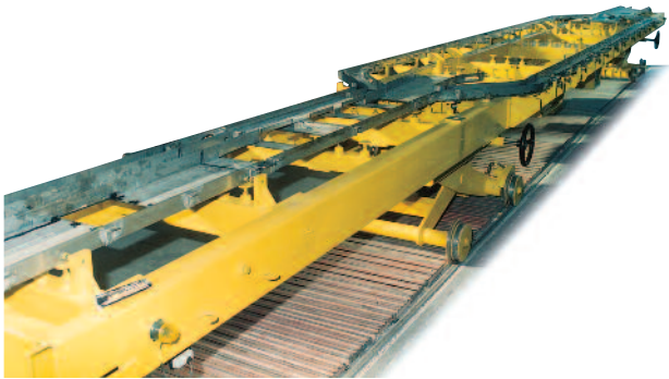
SBA 8R 8,5/4 8,5 t – 19000/23000 x 2000 x 900 (1600) mm Railway electrical conductors handling
