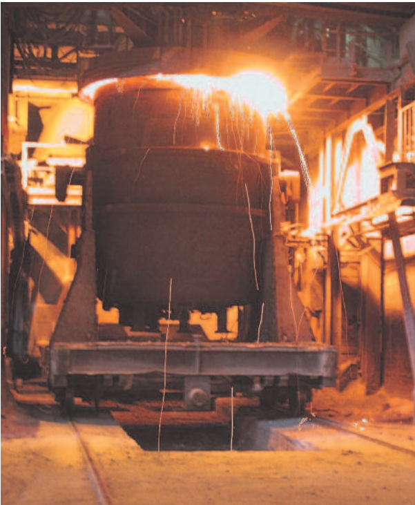
SBR 4R 150/2 Capacity load 150 t Iron ladles handling
