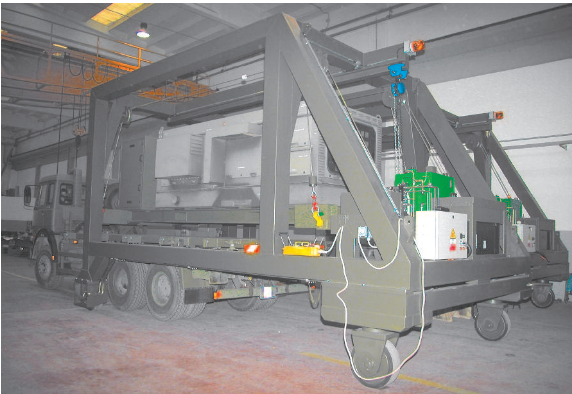
SGAI - VS E 8/2 Capacity load 8 t - Containers 20' translation and lifting
