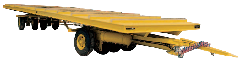
VCP1 30/2 30 t – 12000 x 2500 mm Steel plates handling
