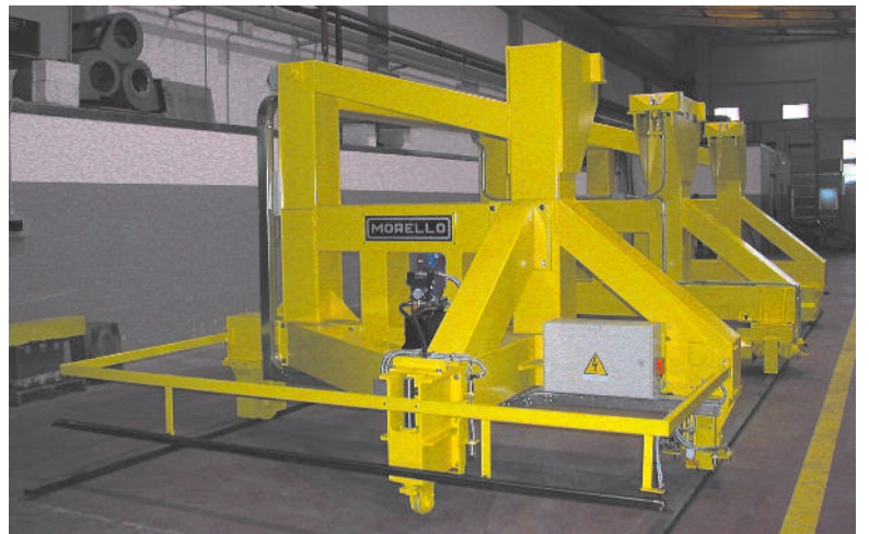
SBR 6R 30/3 special 30 t – 8000 x 3250 mm Coils handling in self-acting mode
