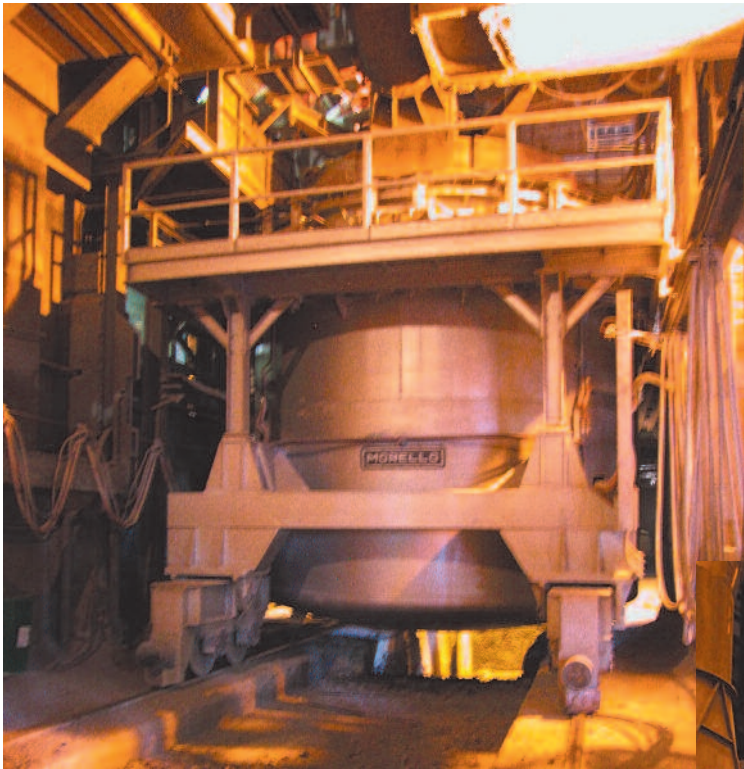
SBR 8R 250/4 Capacity load 250 t Ladles steel mill handling for degassing
