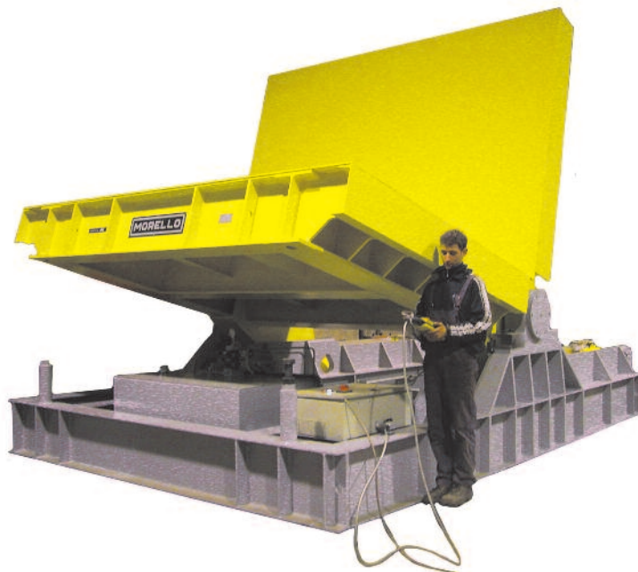
RS 46/90 46 t – 2500 x 2500 x 3000 mm 90° tipper of systems components
