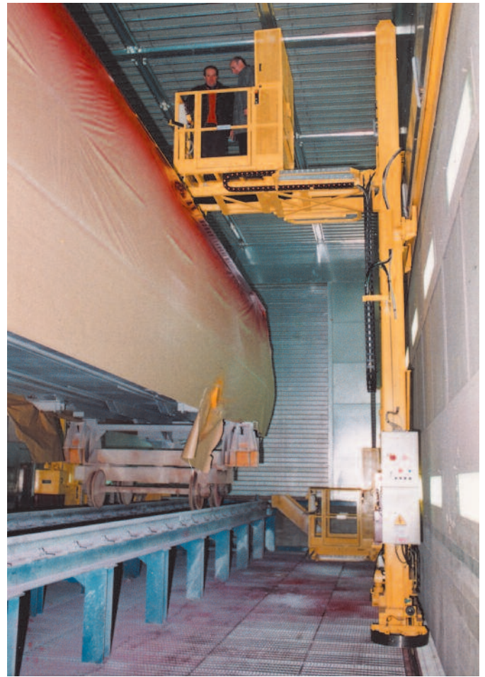
Handling system personnel in painting box Capacity load 300 kg Upstroke 5800 mm Transversal run 2500 mm Longitudinal run 30 m
