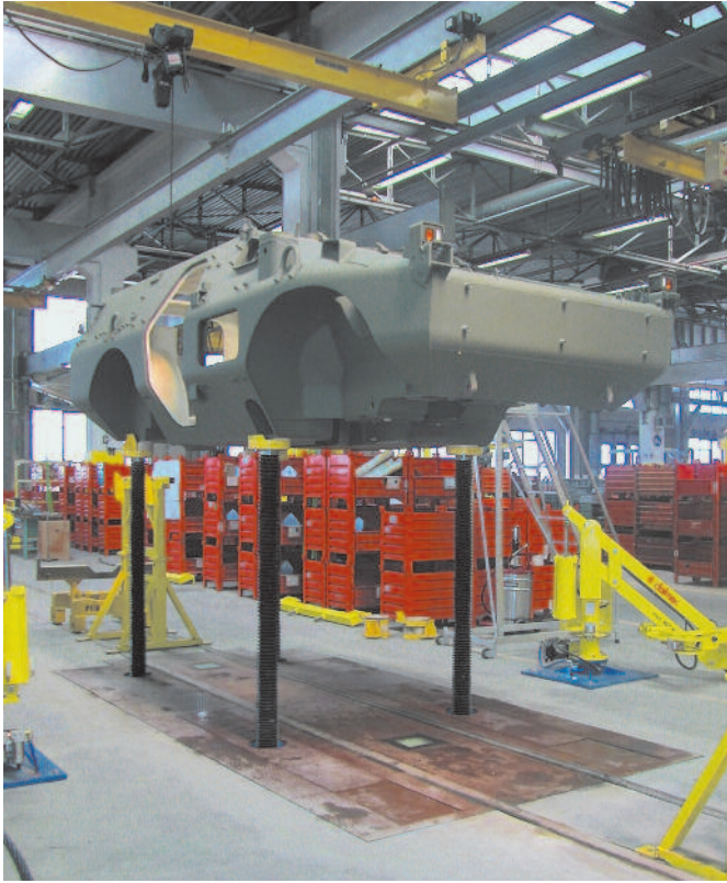
Tired equipments lifting system Capacity load 10 t Upstroke 1800 mm
