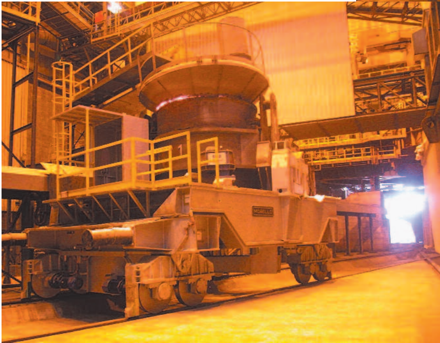
SBR 8R 440/4 Capacity load 440 t with weighing system Ladles steel mill handling
