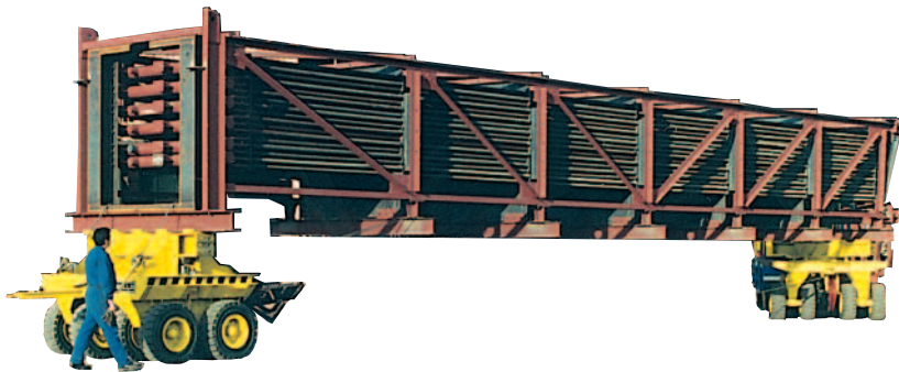
VSP1/R - PI E 120/4 120 t – 2000 + 2000 x 2500 mm Boiler tube bundles handling
