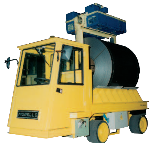
SGAI - VSF 25/2 25 t - 2700 x 1700 mm Coils handling
