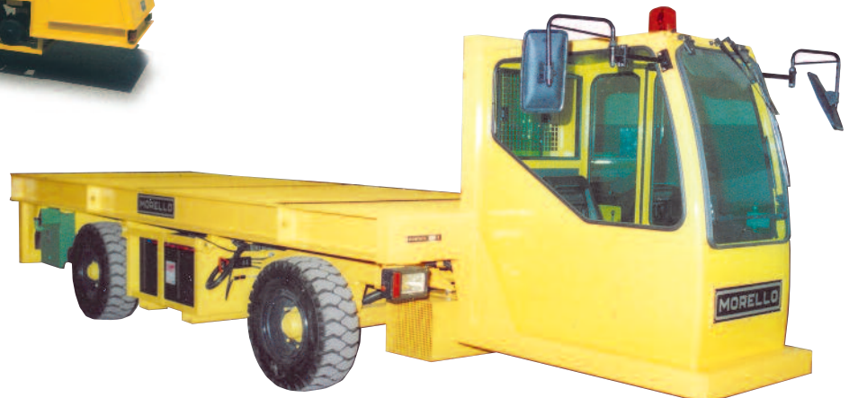
SGAI - VS/VSP1 32/2 32 t - 5750 x 1950 mm Aluminium coils handling
