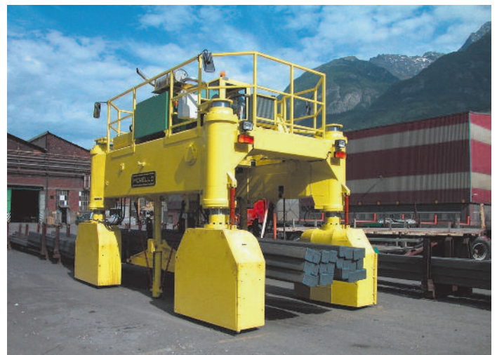
SGD VC E 30/2 Capacity load 30 t Iron and steel products translation and lifting
