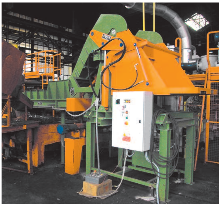
RC 3/180 with conveyor belt 180° tipper for boxes with conveyor belt for pieces scavenging
