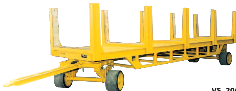
VS 20/2 20 t – 7000 x 1650 mm Steel pipes handling
