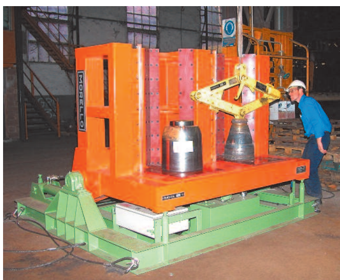
RS 5/90 5 t – 1100 x 1220 x 2250 mm 90° tipper of equipments
