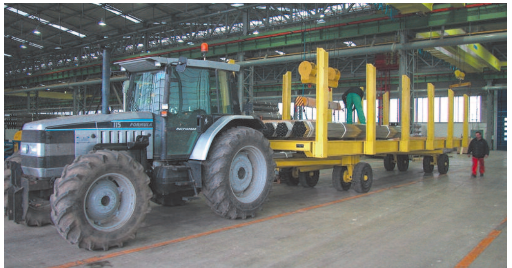
VC/AC 19/3 19 t – 8000 x 2500 mm Naval structures handling
