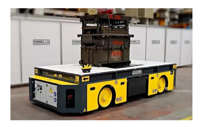
SELF-MOVED ELECTRONIC TRAILER, series SGAE VC R 30/2, operator on ground, for factory material handling on concrete flat and levelled floor
