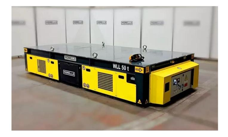
SELF-MOVED ELECTRONIC TRAILER, series SGAE VC P 50/2, operator on ground, for factory material handling on concrete flat and levelled floor
