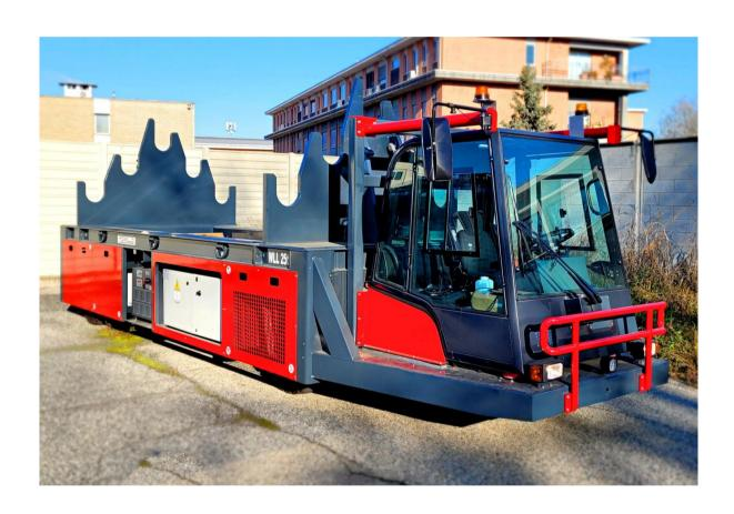
SELF-MOVED ELECTRONIC TRAILER, series SGAI-C VSF I 30/2, operator on board, for factory material handling on concrete and good asphalt, flat and levelled floor
